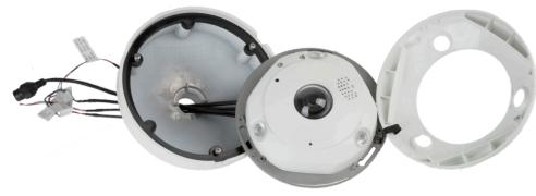
Thread the cables through the cap. Align the camera mounting grooves with the screws, then rotate the camera to lock it into place.
