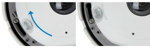
Tighten the mounting screws to secure the camera. Replace the skirt.
