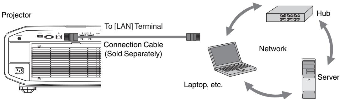
Connect the projector to a network connection device (hub, etc.) via LAN cable.
