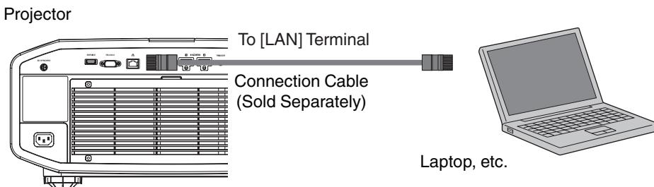
Connect the projector to a PC via LAN cable.
