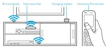
The Harmony Hub can be placed in any unobstructed location where IR signals can be transmitted to AV equipment or it can be placed behind closed cabinets with the IR mini blaster transmitters connected to the hub and positioned as shown above.
