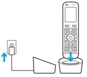
Plug in the charging station and place the remote in it. Keep the remote in the charging station until setup is complete. The charging station should be in the same room as your hub to optimize communication between the remote and the hub.
