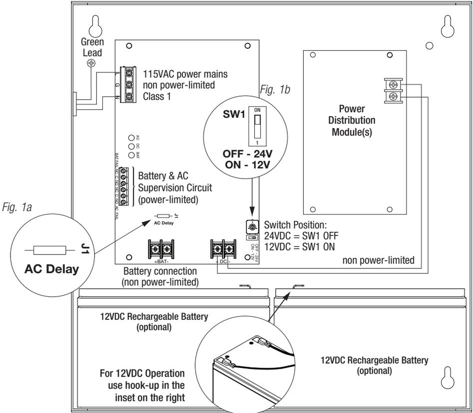
**CAUTION:** When power supply board is set for 12VDC use only one (1) 12VDC stand-by battery. Keep power-limited wiring separate from non power-limited. Use minimum 0.25" spacing.
