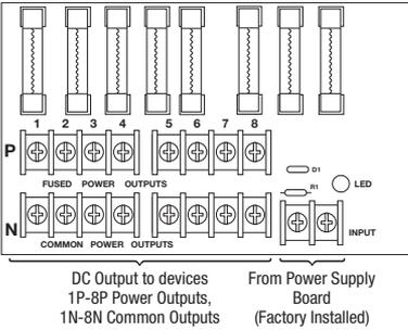
*Fig. 3b* - PD8ULCB Power Distribution Board
