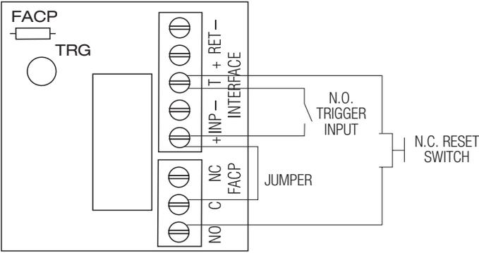
Fig. 7 Normally Closed: Non-Latching FACP trigger input:
