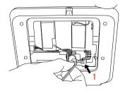
With the included power supply and cable, plug the barrel connector into the barrel jack as shown above.
