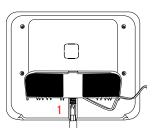
1. With a small phillips screwdriver, screw in the locking screw from the bottom of the panel to secure it to the table stand.
