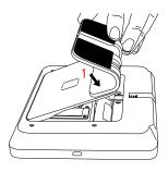
Locate the SmartMount table stand and insert the hooks into the back of the panel, then swing down and press into place.
