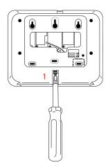
With a small phillips screwdriver, undo the locking screw from the back of the panel, remove the SmartMount backplate and discard.
