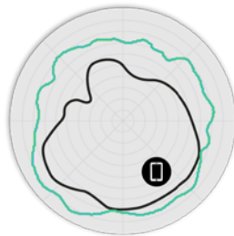
Fig 6. A770 5GHz Elevation Antenna Patterns
