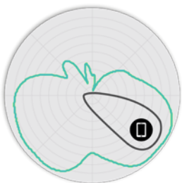
Fig 5. A770 2.4GHz Elevation Antenna Patterns
