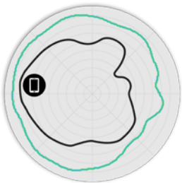
Fig 5. A770 2.4GHz Elevation Antenna Patterns
