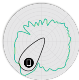
Fig 6. A770 5GHz Elevation Antenna Patterns
