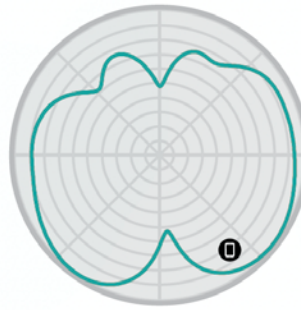
Fig 3. 2.4GHz Elevation Antenna Patterns
