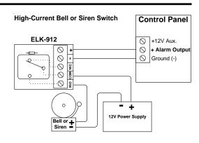
**Example 4:** ELK-912 used to switch a high-current siren or bell from separate power supply.
