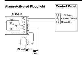
**Example 3:** Floodlight activates whenever control panel is in alarm
