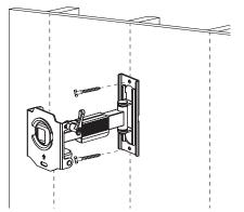
**Warning:** Tighten the screws so that the wall plate is firmly attached, but do not over tighten. Over tightening can damage the screws, greatly reducing their holding strength.
