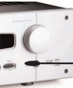
4. Self-adhesive “Flashers” affix to the front panels of your client’s components (over the built-in IR sensor). The Flashers relay commands to components out of sight of the MRF-260’s Front Blaster. The flashers plug in to the MRF-260’s rear flasher line outputs via their 10 foot cables. *Uniquely, the MRF-260 can also connect to rear panel IR Inputs via its two adjustable Outputs.*
