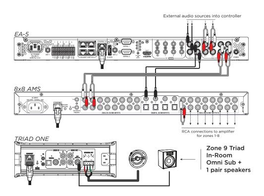
(connect the rest of the 8 zone system as shown in "Connecting an 8 source, 8 zone system")
