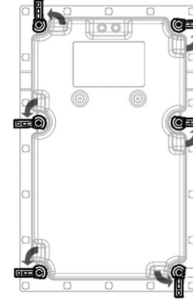
Mounting doglegs will move outward and tighten to secure the speaker to the drywall.
