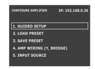
In the AMP WIRING SETUP, verify the Y 1+2 box is NOT checked so inputs will not be combined. The inputs will be combined in a later step. This ensures maximum output of the amp. Leave the BRIDGE box unchecked, highlight the NEXT button and select it.
