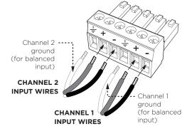
Using the female RCA-to-bare-wire adapter (included with GA Subs), connect wires from channels 1 & 2 into the Phoenix connector as shown at left. Be sure to observe proper polarity when connecting the wires to the Phoenix connector.
