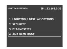
In the AMP GAIN MODE menu, select AMP GAIN. Via the encoder knob, setthe AMP GAIN to +37 dBu and select with the Encoder knob. Select DONE when complete.
