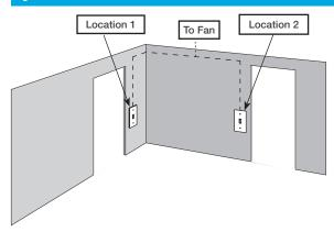
Two switches control the fan (3-way installation)
