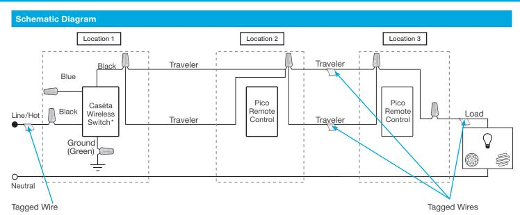
$<sup>^{\</sup>ast}$  It is recommended to install in-wall switch in either Location 1 or 3.
