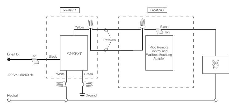
\* Control can be installed in either location.
