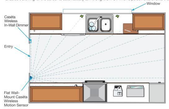
\* DO NOT place sensor within 4 ft (1.2 m) of moving air currents (e.g., HVAC vents), heat source (e.g., light bulbs or microwave/ standard ovens). Heat from an oven may cause sensor to see movement. Changing the activity setting to medium- or high-activity may be necessary. Refer to the back of the sensor or visit:
