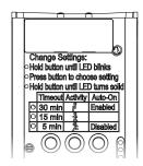
The motion sensor has several advanced set-up features. For the majority of installations, the default settings will provide the best performance and you will not need to utilize the advanced set-up. The motion sensor has three adjustable advanced set-up modes: Timeout, Activity, and Auto-On.
