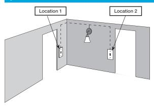
Two switches control the lights (3-way installation)
