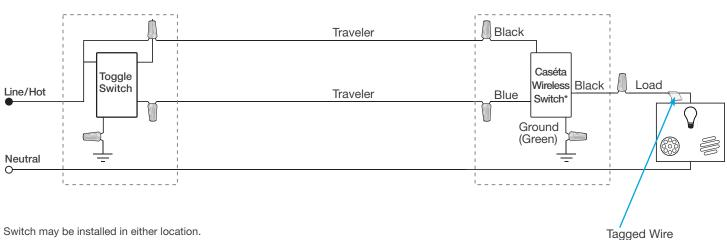
\* Switch may be installed in either location.
