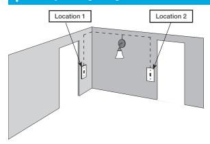
Two switches control the lights (3-way installation)
