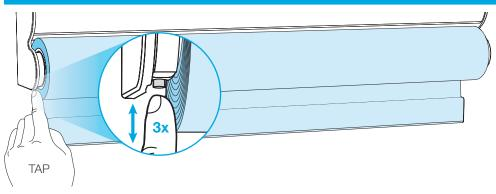
NOTE: The "Shade" button LED will flash GREEN-then-RED three times, signaling the successful completion of the procedure.
