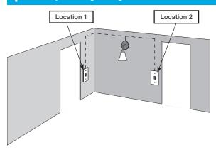
Two switches control the lights (3-way installation)
