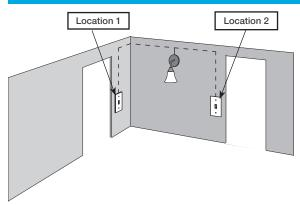
Two switches control the lights (3-way installation)
