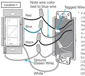
If available, connect the neutral wire from the wallbox to the white wire on the in-wall dimmer. If neutral is not available, cap the white wire with a wire connector. Neutral required for: MLV loads, LED drivers, PHPM-PA, PHPM-3F. GRX-TVI.
