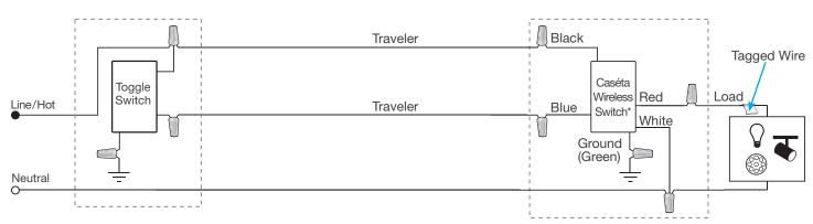
\* Switch may be installed in either location.
