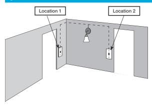
Two switches control the lights (3-way installation)
