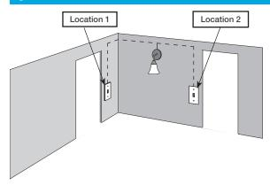
Two switches control the lights (3-way installation)
