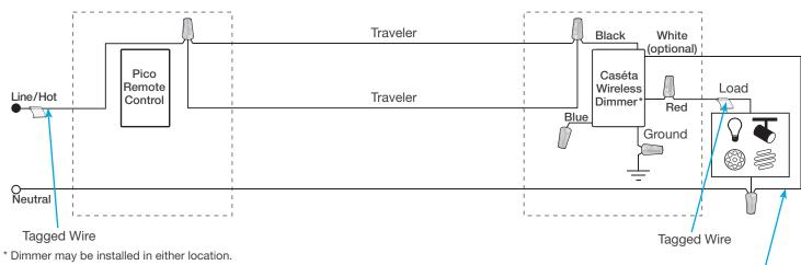
If available, connect the neutral wire from the wallbox to the white wire on the in-wall dimmer. If neutral is not available, cap the white wire with a wire connector. Neutral required for: MLV loads, LED drivers, PHPM-PA, PHPM-3F, GRX-TVI.
