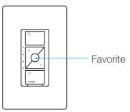
You can use the round "Favorite" button on the fan control to recall a favorite fan speed setting. We've set it to the medium fan speed, but you can change it to any level you like.
