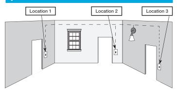
Three or more switches control the lights (multi-location installation)
