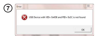
If you receive the following error the matrix has not been connected to the PC through the USB cable. Please check the connection. You will have to start from step 4 with the power off the matrix.
