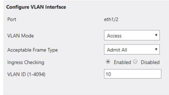
Next, the S3L-24P requires you to create an IP interface for the VLAN where IGMP Snooping can be configured.
