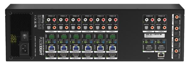
The neo:XMR Video & Audio Matrix - with both audio and video inputs and video and audio outputs. Featuring 6 HDMI inputs, 6 HDBaseT Outputs and 2 HDMI outputs alongside 8 audio output zones (with the options of Stereo L/R, Optical and Digital Coax) and 4 audio input zones (with the option of Optical and Digital Coax).
