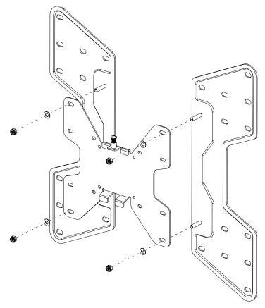
**Note:** The studs on the adapter plate should face away from the TV.
