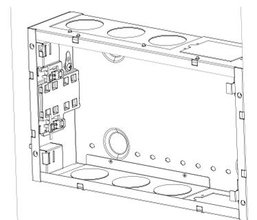
**Note:** You cannot mount vertically in new installs. To mount vertically, the dog ears must clasp the drywall.
