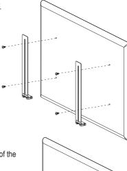
2. Insert the Tray brackets into the rear of the Hook Brackets. Keep the set screws loose to allow for adjusting the depth of the soundbar once installed in step 3.
