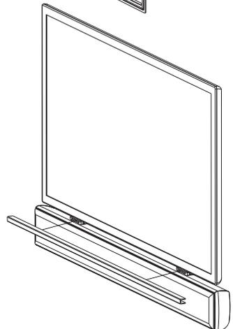
5. Attach the Soundbar to the installed Tray brackets and secure with the screws provided with the Episode™ soundbar.
