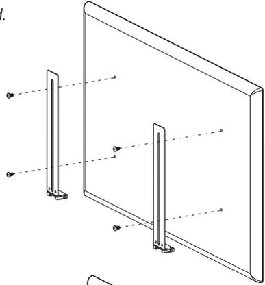
2. Insert the Tray brackets into the rear of the Hook Brackets. Keep the set screws loose to allow for adjusting the depth of the soundbar once installed in step 3.
