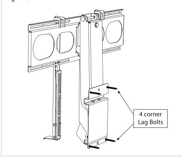
Single Stud Attachment (continued): Only two Lag Bolts are accessible when the Lifting Mechanism (35) is in the UP position. Install one Lag Bolt in the top hole and one Lag Bolt in the bottom slot. Then pull the Lifting Mechanism down and install the Safety Bolt according to the Installation Manual. Install the third Lag Bolt after the Lifting Mechanism is safely locked in the lowered position.
