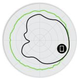
Figure 4. A510 2.4GHz Elevation Antenna Patterns
