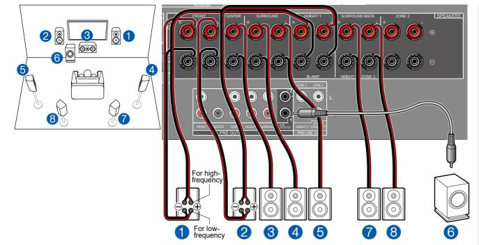
You can configure a 7.1 Channel System ( $\rightarrow p21$ ) by connecting front speakers that support Bi-Amping connection. The Bi-Amping connection can improve the quality of the low and high pitched ranges. Be sure to remove the jumper bar connecting between the woofer jacks and tweeter jacks of the Bi-Amping supported speakers. Refer to the instruction manual of your speakers as well. ■ "Speaker Setup" settings during Initial Setup ( →<u>p183</u>)
