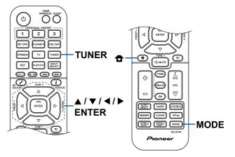
When FM broadcasts reception is poor: Perform the procedure for "Tuning Manually" ( $\rightarrow p111$ ). Note that if you tune manually, the reception for FM broadcasts will be monaural rather than stereo, irrespective of the sensitivity of the reception.
