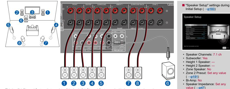
This is a 7.1 Channel System that consists of the basic 5.1 Channel System and added surround back speakers. For details of the speaker layout, refer to "Speaker Installation" ( $\rightarrow p21$ ).
