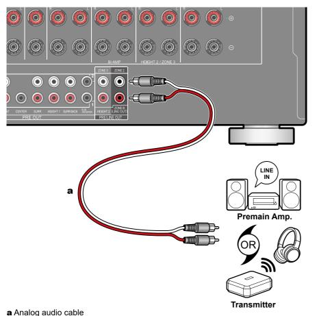
While performing playback through speakers (ZONE A) connected to the unit, you can enjoy the audio of the same source at the same time with the pre-main amplifier or the transmitter of the wireless headphones connected to the ZONE B LINE OUT jack. Use an analog audio cable to connect the ZONE B LINE OUT jack of this unit and the LINE IN jack of the pre-main amplifier or the transmitter of the wireless headphones.
