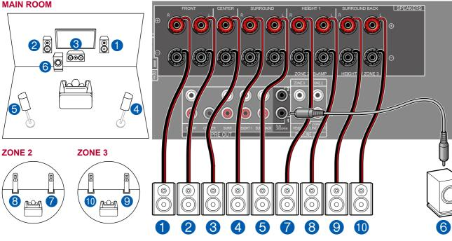
**MAIN ROOM:** This is a basic 5.1 Channel System. For details of the speaker layout, refer to "Speaker Installation"  $(\rightarrow p20)$ .
