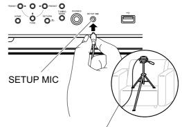
When placing the speaker setup microphone on a tripod, refer to the illustration.
