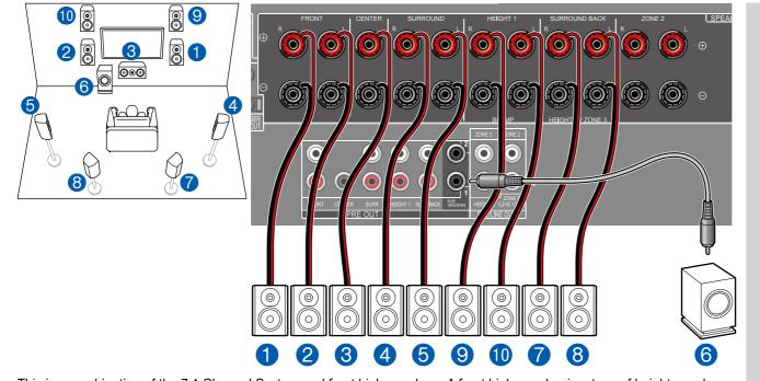
This is a combination of the 7.1 Channel System and front high speakers. A front high speaker is a type of height speaker. You can select only one set of height speakers from the following three types for connection.
