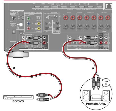
You can enjoy 2-ch audio in the separate room (ZONE 3) while performing playback in the main room (where this unit is located). Use an analog cable to connect the ZONE 3 PRE/LINE OUT jack of this unit and the LINE IN jack of the pre-main amplifier or power amplifier in the separate room. The same source can be played back in the main room and ZONE 3 simultaneously. Also, different sources can be played back in both rooms.
