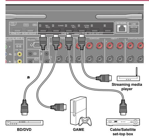
This is a connection example of an AV component equipped with an HDMI jack. When connecting with an AV component that conforms to the CEC (Consumer Electronics Control) standard, you can use the HDMI CEC function (\*) that enables linking with input selectors, etc. and the HDMI Standby Through function that can transmit video and audio signals of the AV component to the TV even if this unit is in standby mode.
