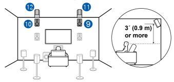
The width between the rear high speakers should match the one for the front speakers, and they should be installed minimum of 3'/0.9 m higher than the front speakers, and tilted so they will point toward the listener.
