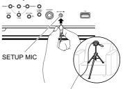
When putting the speaker setup microphone on a tripod, refer to the illustration when putting it in place.
