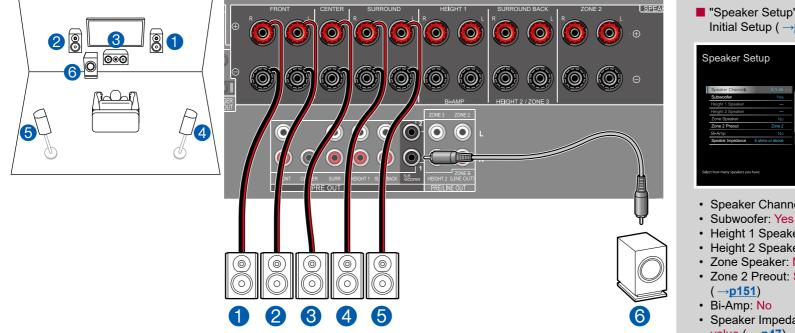
This is a basic 5.1 Channel System. For details of the speaker layout, refer to "Speaker Installation" ( $\rightarrow p20$ ).
