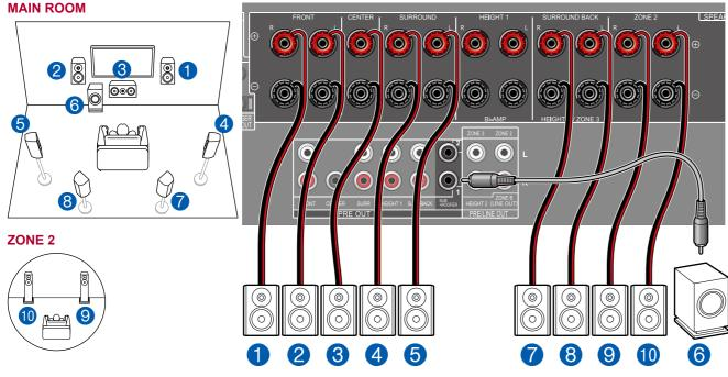
**MAIN ROOM:** This is a 7.1 Channel System that consists of the basic 5.1 Channel System and added surround back speakers. For details of the speaker layout, refer to "Speaker Installation" ( $\rightarrow p21$ ).
