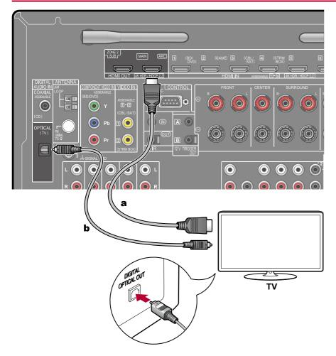
If the TV does not support the ARC (Audio Return Channel) function (\*), connect an HDMI cable and digital optical cable.
