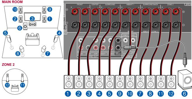
**MAIN ROOM:** This is a combination of the 7.1 Channel System and front high speakers. A front high speaker is a type of height speaker. You can select only one set of height speakers from the following three types for connection.
