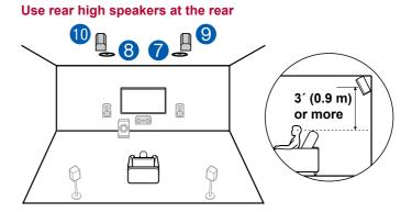
The width between the rear high speakers should match the one for the front speakers, and they should be installed minimum of 3'/0.9 m higher than the front speakers, and tilted so they will point toward the listener.
