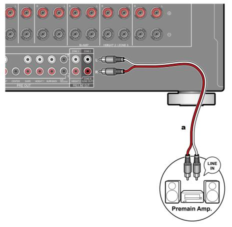
You can enjoy 2-ch audio in the separate room (ZONE 2) while performing playback in the main room (where this unit is located). Connect the ZONE 2 PRE/ LINE OUT jacks of the unit and the LINE IN jacks of the pre-main amplifier or power amplifier in a separate room with an analog audio cable. The same source can be played back in the main room and ZONE 2 simultaneously. Also, different sources can be played back in both rooms.
