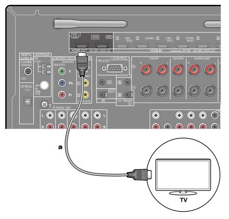
While a disc is played on a Blu-ray Disc player in the main room (where this unit is located), you can play the video and audio of the same Blu-ray Disc player or another AV component on the TV equipped with an HDMI IN jack in a separate room (ZONE 2). The TV in the separate room can play only the video of devices connected to the HDMI IN1 to IN3 jacks of this unit.
