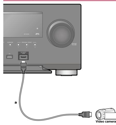
Connect a video camera, etc. to the AUX INPUT HDMI jack on the front panel using an HDMI cable.
