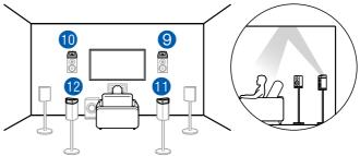
The Dolby enabled speakers are the special speaker that the sound is emitted toward the ceiling, and have the effect the sound to come from above by reflecting the sound on the ceiling.
