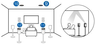
The Dolby enabled speakers are the special speaker that the sound is emitted toward the ceiling, and have the effect the sound to come from above by reflecting the sound on the ceiling.
