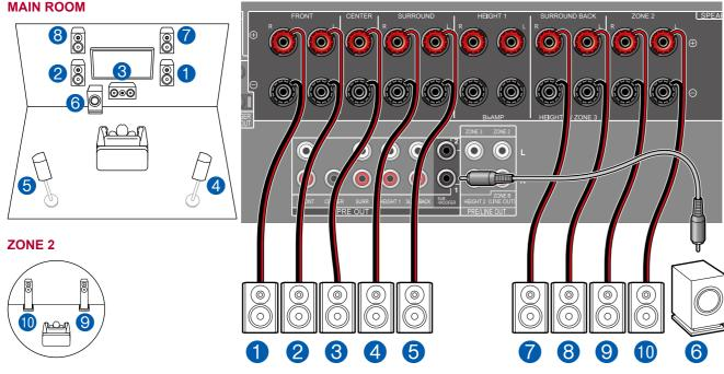
**MAIN ROOM:** This is a combination of the 5.1 Channel System and front high speakers. A front high speaker is a type of height speaker. You can select only one set of height speakers from the following three types for connection.
