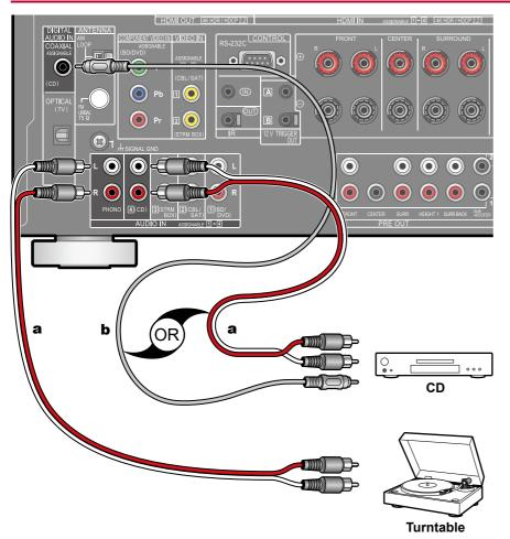
This is a connection example of an audio component. Connect a CD player using a digital coaxial cable or analog audio cable. You can also connect a turntable that has an MM-type cartridge to the PHONO jack.
