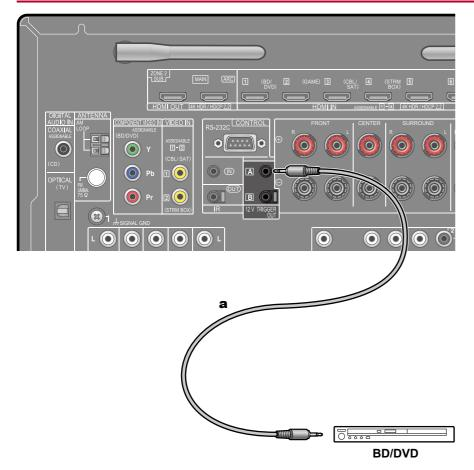
When connecting a device equipped with a TRIGGER IN jack such as a BD/DVD player to this unit, the device can be turned on or set to standby by interlocking the operation on this unit. When the desired input is selected on the unit, power link operation will be activated with a control signal of maximum 12 V/100 mA from the 12V TRIGGER OUT A jack or maximum 12 V/25 mA when using the 12V TRIGGER OUT B jack. You can select the zone to output the control signal by setting each of the inputs.
