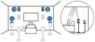
The Dolby enabled speakers are the special speaker that the sound is emitted toward the ceiling, and have the effect the sound to come from above by reflecting the sound on the ceiling.
