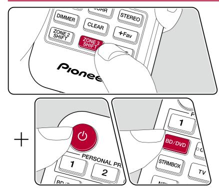
In the remote controller operation, while pressing and holding the ZONE 3 SHIFT button on the remote controller, operate with each button. Settings are required to playback a source in ZONE 3.
