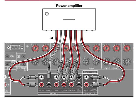
You can connect a power amplifier to the unit and use the unit as a pre-amplifier in order to produce a large volume that cannot be output with the unit only. Connect the speakers to the power amplifier. For details, refer to the power amplifier's instruction manual.
