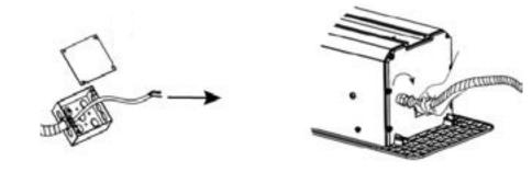
3. Position and mount the attached power junction box. Do not kink the flexible conduit during installation.
