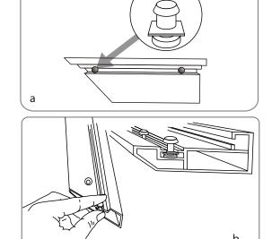
• The snap lugs line up with the arrow decals on the frame tubes. Alignment is not critical at this stage of the installation. Note that the screen is supplied with 2 extra snap lugs; should you lose or break a snap lug, one of the spares is a convenient replacement.
