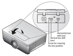
Suggest to loosen the screw before lens shift adjustment and tighten up after finished adjustment.
