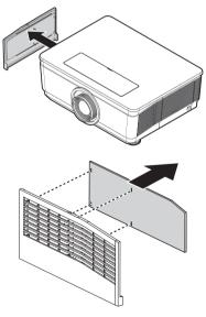
3. Replace a new filter module or replace filter into cover.
