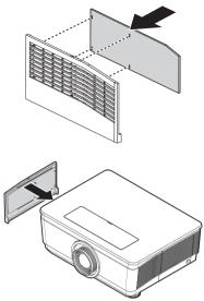
4. Replace the filter cover back to the projector by pushing gently in the direction shown.
