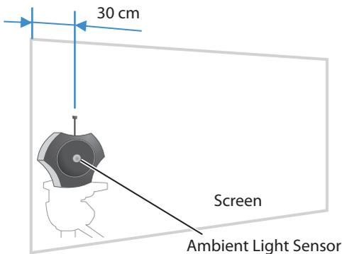
Position the optical sensor at approximately 30 cm from the edge of the projected image with it in contact with the screen, and make sure the ambient light sensor is facing the projector.
