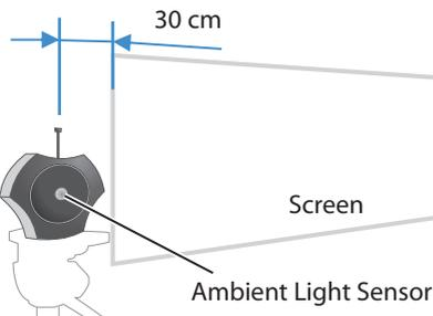
When measuring the intensity of ambient light, place the optical sensor parallel to the screen at a position where light from the projector does not fall directly on the optical sensor (approximately 30 cm away from the edge of the projected image). At the same time, make sure the ambient light sensor is facing the projector.
