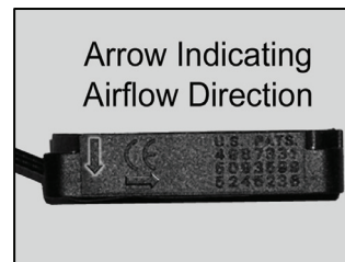
Figure 3: Check airflow direction
