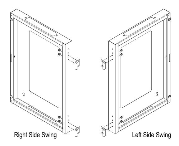
**E.** Insert the Hinge Pins into the Hinge Plates on the swing kit and secure with the set screw.
