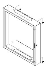
**G.** Slide the rack onto the Hinge Plates and Pins mounted to the Swing Assembly.
