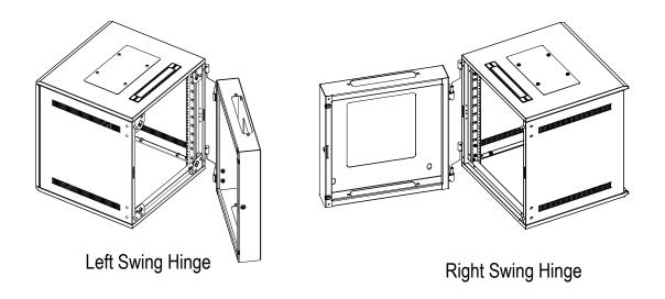
**H.** Secure the hinges with the set screws.
