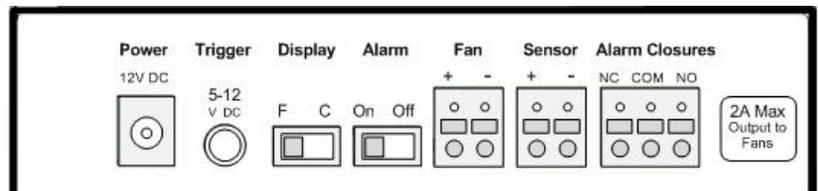
**Fan:** This is the connectors for the fan/s. For Cool Components products, use the supplied fan cable and connect the wire with the white stripe to positive (+). For other fan units, ensure connection is correct as not all fans are polarity protected and damage may occur to the fan (All CCI fans are protected, fans from other manufacturers may not be).
