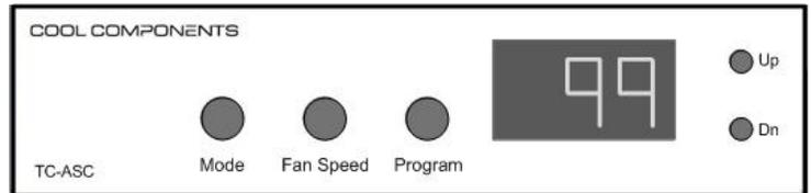
**Mode:** This is to determine if the unit will function automatically based on temperature or turn on and off based on the low voltage trigger. To change the setting, simply press the button until the desired setting is displayed. The image to the right translates each setting with what is displayed on the screen to the right.
