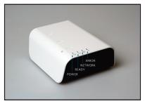
**Power LED:** Illuminates to indicate the TRF-ZW1 is powered.
