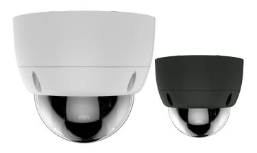
The ClareVision 4MP Motorized Varifocal IP Dome Camera features the Sony® Starvis™ sensor with a 2.7-13.5 mm motorized varifocal lens with autofocus. Additionally, the Dome includes advanced motion detection capabilities which includes line crossing, loitering, and human body detection, as well as a powerful night vision sensor capable of illuminating objects up to 30 meters away.
