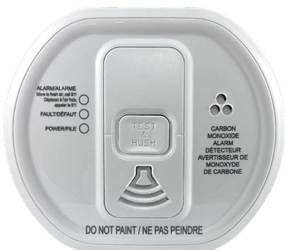
The ClareOne Carbon Monoxide Detector is a battery powered wireless detector that communicates with the ClareOne Panel. The detector consists of an electrochemical CO sensor and a wireless transmitter.
