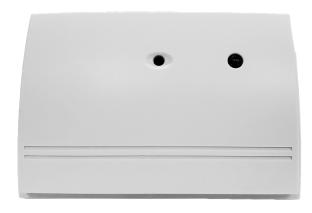
The ClareOne Glass Break Detector detects the shock and sound of breaking glass and sends an alert to the ClareOne Panel. The detector provides a 20 ft. maximum detection range, and can sense sound in a 360° pattern when mounted on a ceiling.
