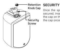
Once the speaker is in the desired position and secured, insert the included safety screw. Remove the cap on the retention knob to access it. Replace the cap once the security screw is tightened.
