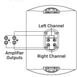
The ES-500-AW-DVC-6 has two sets of terminals (one for each channel). Each input is 8 ohms and a receiver or amplifier capable of 8 ohms speaker load must be used. Connect the Left channel to one set of terminals and the Right channel to the other set.
