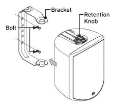
The ES-AW-X speakers are supplied with a U-shaped wall mounting bracket that can be installed vertically, horizontally or under eaves. Use screws, bolts, or anchors (not included) that are capable of supporting the weight of the speaker (see illustration) to mount the bracket.
