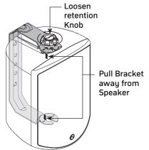
To remove the speaker from the bracket, loosen both retention knobs on the sides of the speaker. Pull the bracket away from the top and bottom of the speaker and then slide the speaker from the bracket
