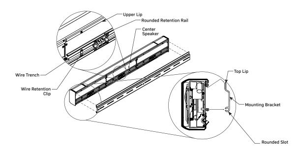
6. Position the center speaker in the center of the rail using the vertical marks on the bracket for guidance. Once the center speaker is in place, position the left and right speakers on the rail following the same steps as above.
