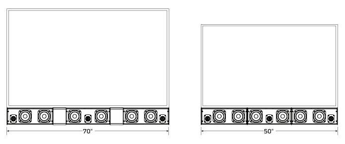
To maintain a high level listening experience, the soundbar should be as close to the TV as possible. Keep in mind when installing the soundbar that placing the soundbar more than 3" from the screen will separate the audio from the video and provide a poor viewing and listening experience.
