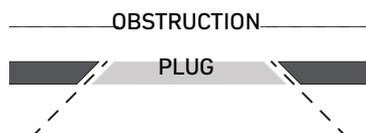
1. Cut the drywall at a 45° angle so that if the speaker is too close to an obstruction, you can easily 'plug' the hole.
