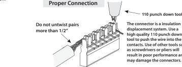
The connector is a insulation high quality 110 punch down tool to push the wire into the contacts. Use of other tools such as screwdrivers or pliers will result in poor performance and may damage the connectors.
