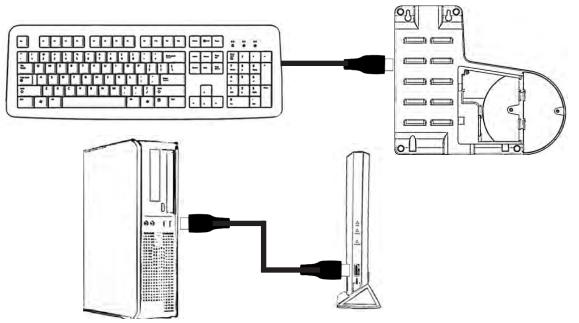
Now use a female-to-female USB cable to connect the USB jack on the transmitter to any USB input on the computer. The USB device connected to the transmitter should now be able to operate the connected computer through the wireless link.
