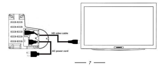
Connect the included 15-foot HD cable to the HD jack on the underside of the receiver. Connect the other end to one of the HD inputs on the TV. Turn on the TV and select the HD input you used to connect the receiver.
