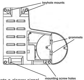
possible, mount the receiver a couple of feet above the TV so it gets a clearer signal.
