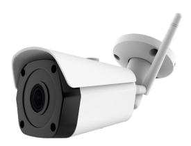
This 4MP Value Series Bullet camera includes Wi-Fi support, allowing for wireless connectivity to the home network. The camera features a 3.6 mm lens that supports a maximum recoding resolution of 2560 x 1440 at 30 FPS. The camera is capable of capturing incredible detail in even the most poorly illuminated areas with IR night vision up to 25 meters, DWDR support, and minimum illumination capabilities at 0.01 LUX.
