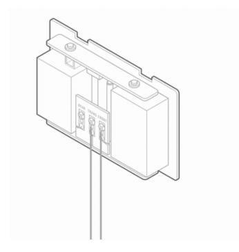
**Note**: The power module must be used in every installation regardless of the chime type. The power module is used to prevent the chime from buzzing or humming, and it helps ensure sufficient power is provided to the Alarm.com Video Doorbell.
