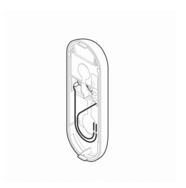
5. Crimp the two wires coming through the backplate to the existing wires threaded through the mounting bracket.
