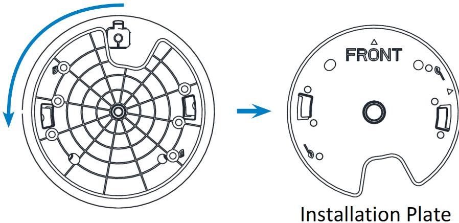
5. Flip the base plate over and attach it to the ceiling as shown.
