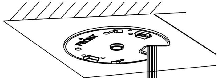
7. Align the PTZ camera with the base plate. Insert the PTZ camera and rotate it clockwise into the base plate until the camera can turn no further (this is the opposite of step 1). Note the icons on the side of the PTZ to ensure you rotate it properly.
