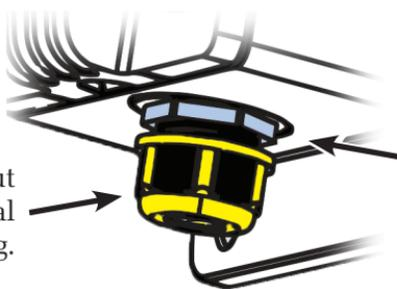
The thin nut secures the connector to the wall box.
