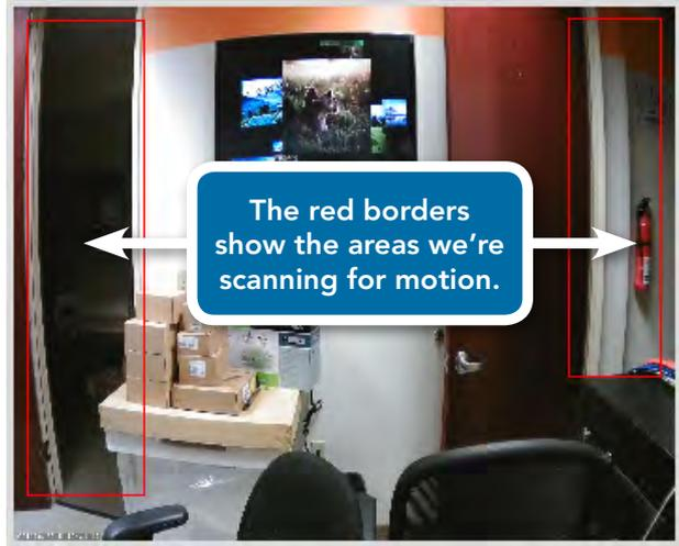
We deliberately left the center of the screen without motion detection, because (a) the TV screen is always “moving,” and (b) if someone is sitting in the chair, we don't want them endlessly triggering motion events.
