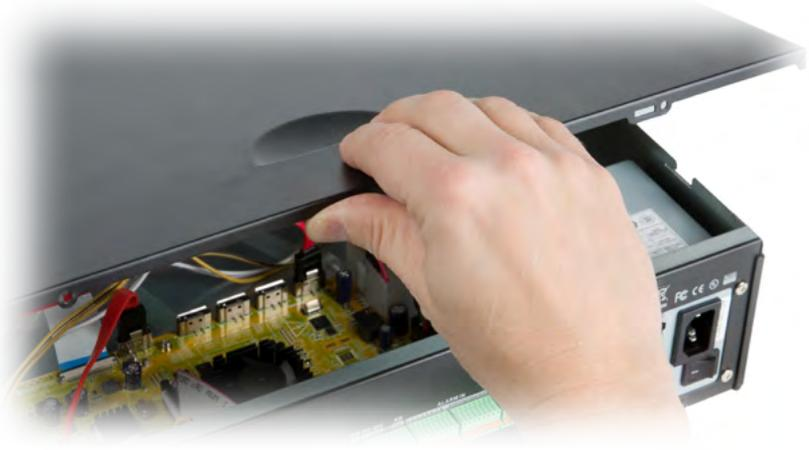
Using the thumb notch on the top of the unit, gently slide the cover about an inch to the rear of the unit, then lift it up. Once it is off, set the lid aside in a safe place where it won't get scratched.
