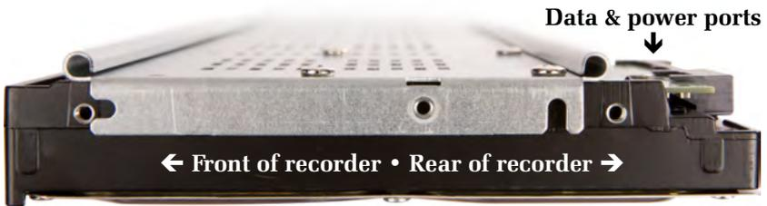
If you removed the old hard drive, look at the side of the mounting bar. The groove that points down should be at the end with the power and data ports, toward the rear of the recorder.
