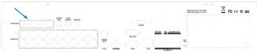
If you have an 8- or 16-channel DVR, and none of the installed cameras has a microphone built in or directly connected, you can attach an external microphone to each of the DVR's four AUDIO IN ports. These four ports correspond **directly and specifically** to channels 1 through 4 of the DVR. Thus, the microphone attached to the second AUDIO IN port can be heard on channel 2. Be sure each microphone's associated camera is on the same channel.
