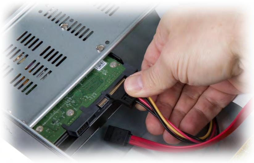
Toward the front of recorder is the mounting bar, a ventilated strip of metal. One hard drive is already installed. Disconnect the SATA and power cables from that hard drive.
