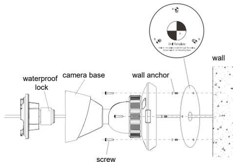
Using the adhesive template, drill 4.5mm holes for the wall anchors (marked B on the template). If needed, drill a hole for the cabling (marked A). If the cabling will run along the wall, mount the camera to a junction box.
