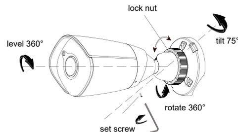
Attach the camera to the base by aligning the unlocked icons on the housing and base, then twisting until the locked icons align. Adjust the camera's aim, then tighten the set screw and lock nut.
