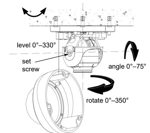
Secure the dome cover to the camera, Remove the protective covering from the dome.
