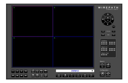
Video images can be displayed in several types of split-window screens including 1/4/9-Window options for a single DVR and 16/25/36/49/64 options if connected to multiple DVRs.
