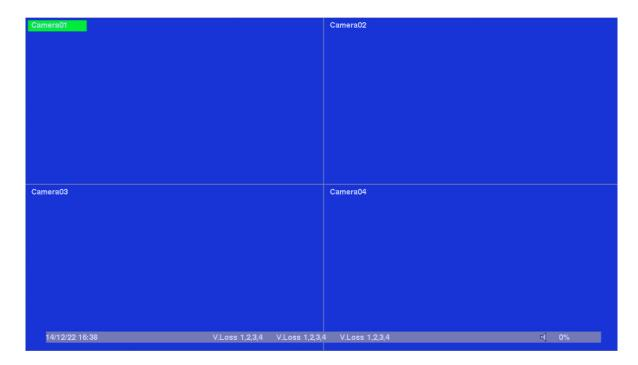
The split-window screen is the main screen displayed after system startup. There are several types of split-window screens including 1 or 4 window grids (as described in **Section 4.3**). In addition to the split windows, a **System Status Bar** is displayed at the bottom of the screen. Time is displayed in the lower-left corner while system status is displayed in the lower-right corner. Scrolling screen messages are displayed when certain events occur.
