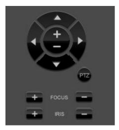
For more control, display the PTZ Control Panel by clicking on the PTZ Panel icon. Move the panel by clicking and dragging the panel to the desired location.
