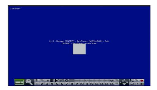
In the **Motion Area Setting** screen use the **white** mask window to define the **Smart Search** area in the same manner as setting up **Motion Detection** (see **Section 6.2.2**).
