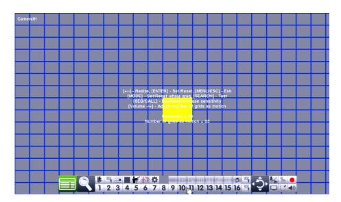
Note: The defined detection area and sensitivity are also used for the **Smart Search** feature (**Section 8.3**). Smart Search will only use information stored "inside" of the detection area. There will not be any motion information stored by the DVR that is "outside" of the detection area. Even if motion detection is disabled for a given camera, it is recommended to enable the entire area if the **Smart Search** feature may be used.
