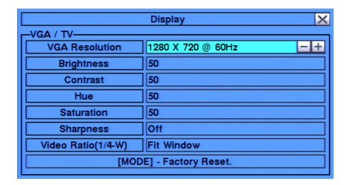
Use the operations listed below to adjust Resolution, Brightness, Contrast, Hue, Saturation and Video Ratio.
