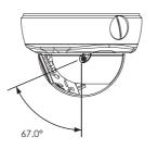
b. After adjustments are made, open and insert the spare silica pack behind the gimbal, then close the camera dome and tighten the screws. Avoid pinching the dome retention wire in the gasket.
