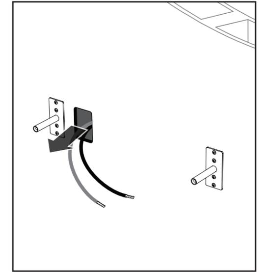
**5** Pull wires through opening in wall.
